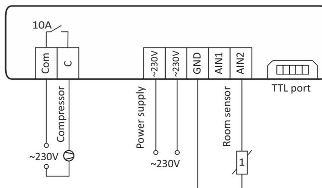
and probe wires is 30 mm. Analog inputs of controller are made for connecting probes of appropriate types only.
